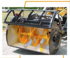
**Bag Opener Spikes** Built into the cover to speed up the loading process.
